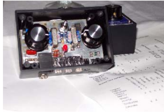
The Sound Card Interface with the top cover removed
